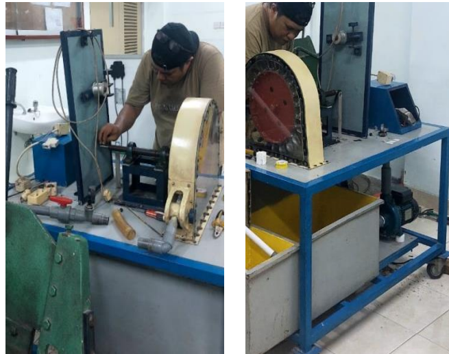
Figure 2. Disassembly of the bucket
