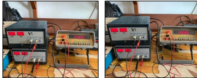
Figure 9. Voltage and Current Measurement Setup Using DC Power Supplies and Digital Multimeter
